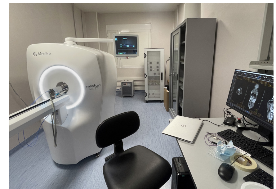
nanoScan® MRI 7T reference installation with every system component (magnet, workstation, electronic cabinet, He-compressor, chiller) located in the same imaging room.
